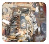
Now the real work begins. The radiator was dust. A blown head gasket spelled disaster for the pistons and it all had to be rebuilt. **TaDaaa...** in sweeps our other hero, *uncle Heikki!*
