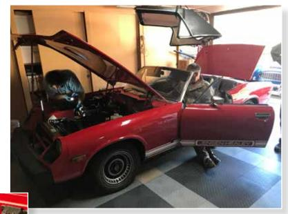
By the end of the session the fuel pump problem was solved, With a new one. The carb intake ducting straightened out, and the steering column key lock was working with judicious key-work. It seems that the brass tumbler bushing was worn and in need of additional work, beyond what the tech session could accomplish. The key would turn and the car would start with said judicious jiggling.
